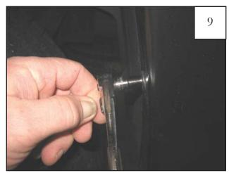
Holding flare in position on fender, reinstall factory screws removed in Step 8.
