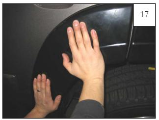
Apply firm pressure to taped areas for proper bond. Tape reaches maximum adhesive bond after 24 hours of contact. Do not wash vehicle until 24 hours have passed.
