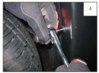
Reinstall factory screws removed in Step 1.
